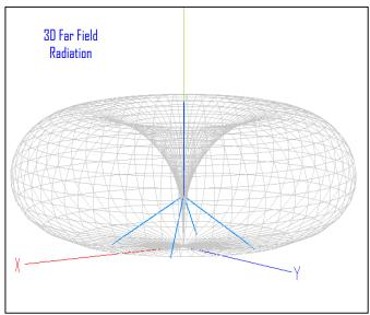
40m Model base :-Radiating element 10.4m long & 1.4 m above ground. The 4 radials 10.62m long & ends 0.4 m above ground. 30m Model base :-Radiating element 7.03 m long & 4.5 m above ground. The 4 radials 7.03 m long & ends 0.7 m above ground. Ground modelled as "REAL" 5ms/m and 13.0 dielectric – i.e. average ground
