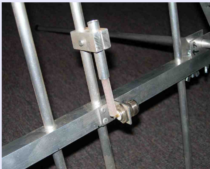
Direct connection to N Socket for 436MHz
