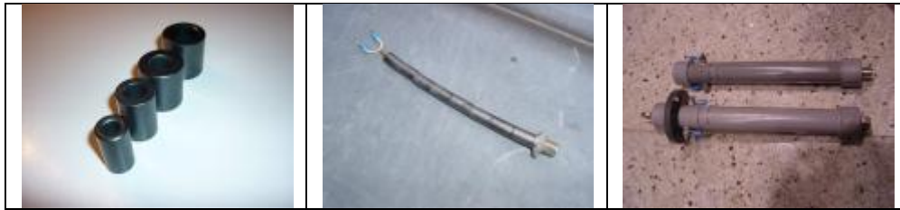
Figure 3. The W2DU current balun: the ferrite beads, the string construction and a waterproof enclosure.
