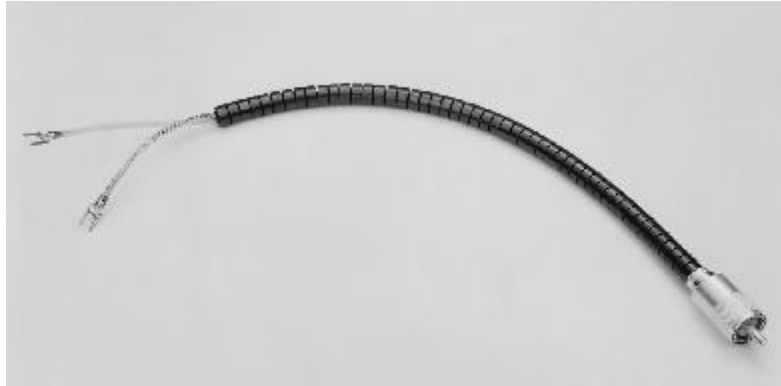
Figure 2. The W2DU current balun
