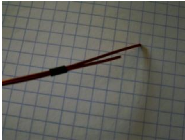
Figure 9b. A trick to identify the specific wire by making it a bit longer at both ends
