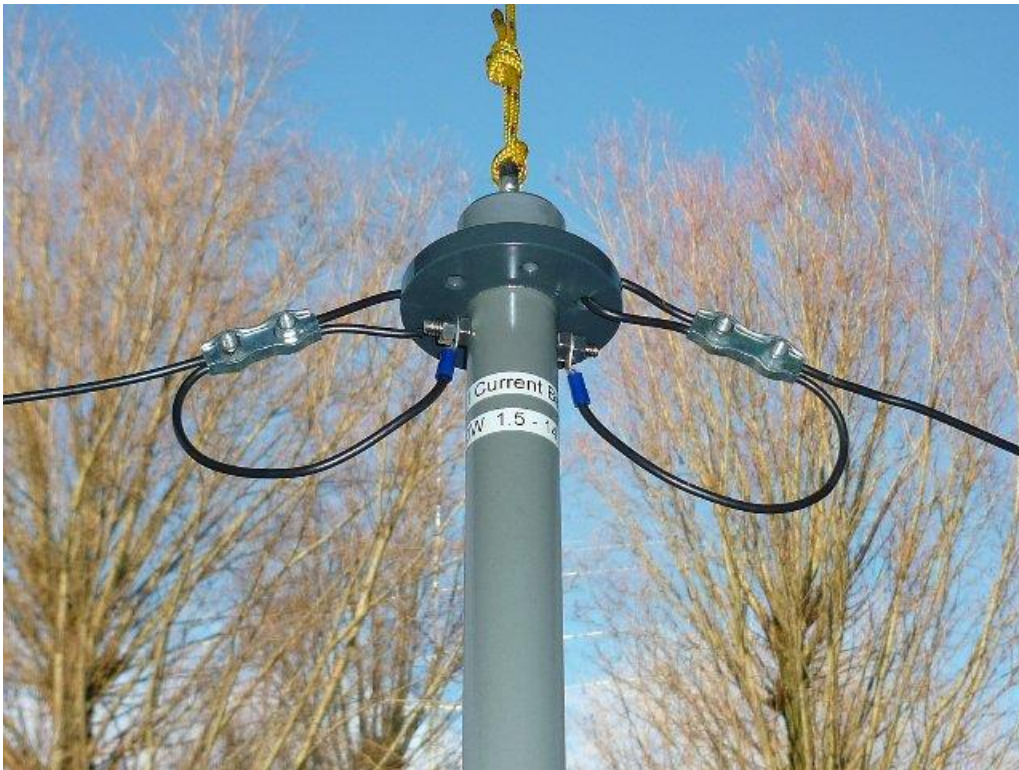
Figure 4. A W2DU current 1:1 balun waterproof construction for use at wire dipole feedpoint
