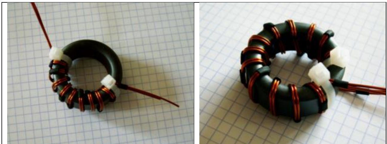
Guanella 1:1 balun wound on one half side of the core. Input and output on opposite side.
