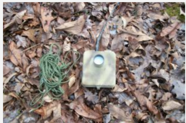
The Dakota Alert, painted and rigged with a homemade rubber duck antenna cut for the MURS frequencies.
